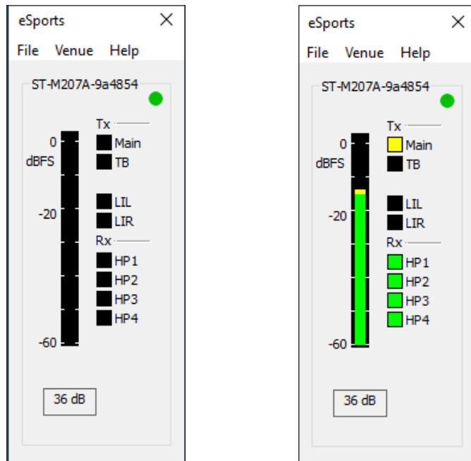
Model 207A eSports Console VenueView showing 'Idle' (left) and 'Active' (right) Screens
