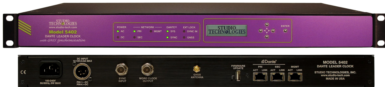
Figure 1. Model 5402 Dante Leader Clock with GNSS Synchronization front and back views
