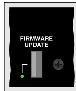
Figure 9. Detail of Model 5418 back panel showing firmware update USB receptacle
