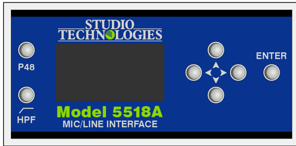
Figure 8. Detail of Model 5518A front panel showing monitor section
