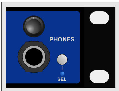
Figure 6. Detail of Model 5518A front panel showing headphone output
