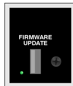
Figure 9. Detail of Model 5518A back panel showing firmware update USB receptacle
