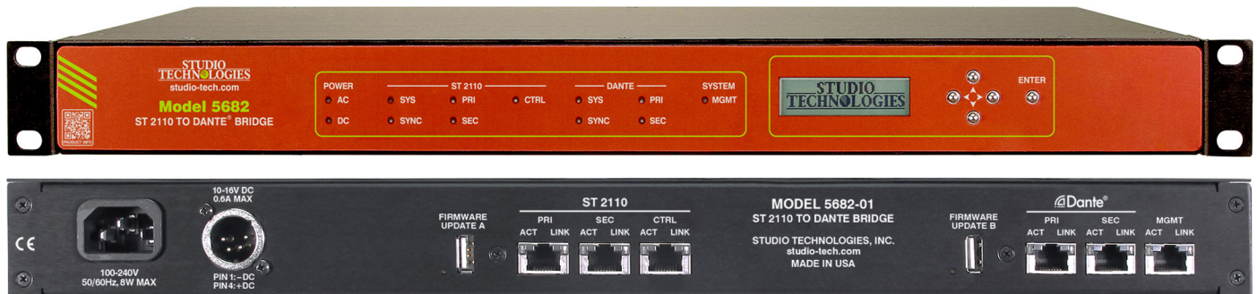
Model 5682 Front View (top) and Model 5682-01 Rear View (bottom, typical for Model 5682-02)
