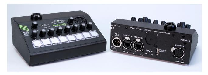
A Dante receiver (input) channel can also be used as a talk audio source. This was specifically included to allow two Model 348 units to "work" together to support more than eight talk channels. A pushbutton switch allows users to directly select the active talk audio source. Choices include the headset mic, the gooseneck mic, or the Dante Aux In receiver (input) channel.
