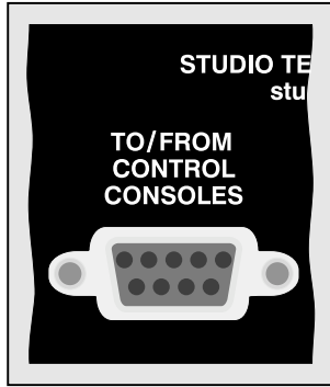
Figure 13. Detail of Model 792 back panel showing the DE-9F connector
