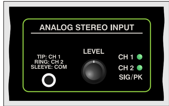
Figure 11. Detail of Model 792 front panel showing analog stereo input
