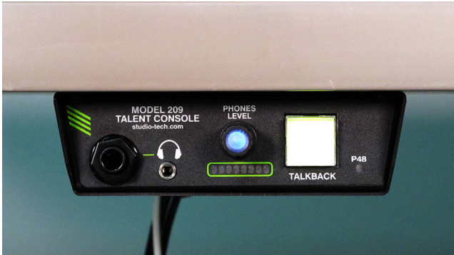
Figure 2. Model 209 Talent Console shown in an under-tabletop mounting configuration
