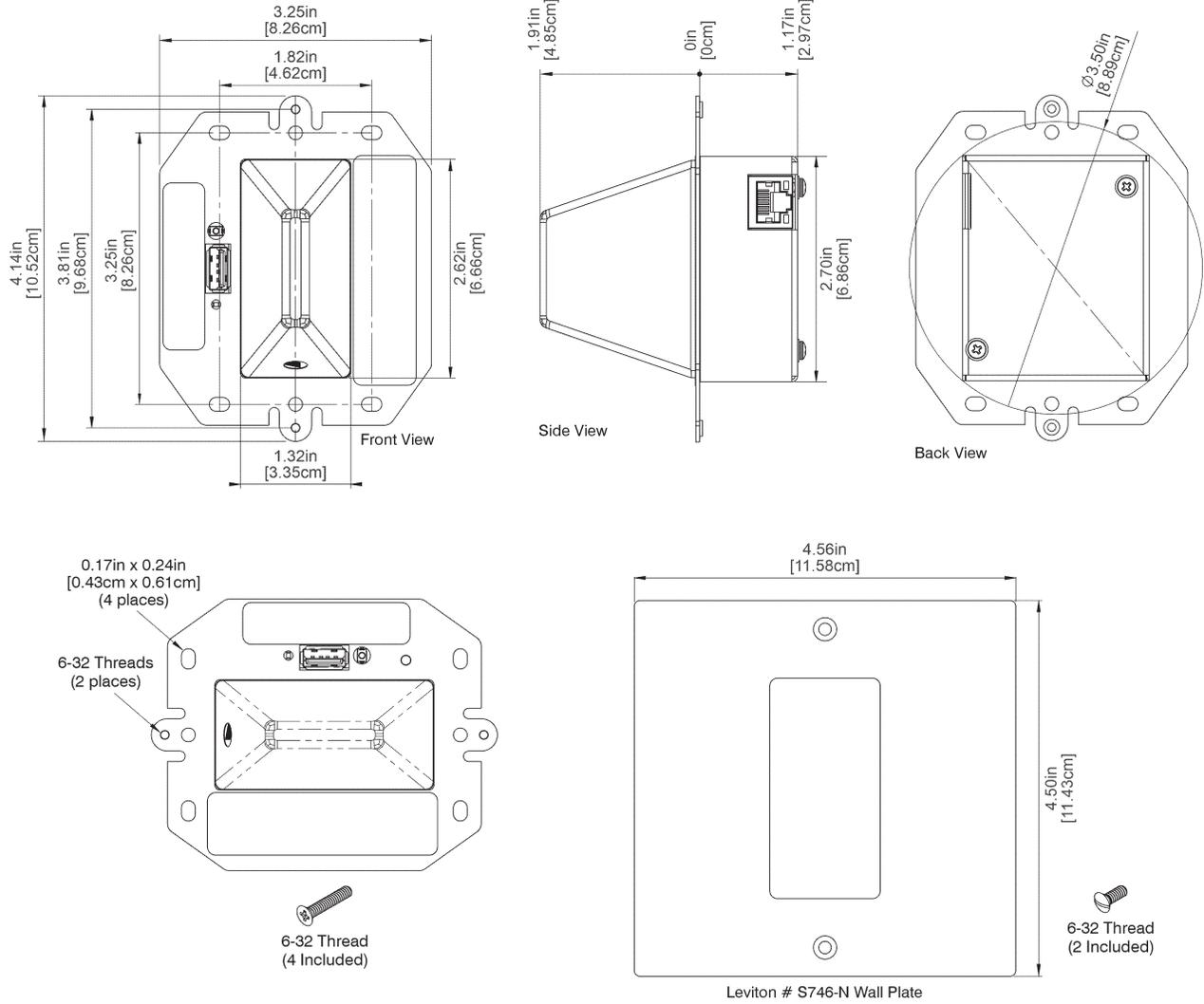
Recommended for use with any commercial electrical box, low-voltage device box, or suitable panel/drywall mounting bracket in a 2-gang configuration. Recommended for horizontal or vertical wall mounting as shown. May also be mounted to ceilings. Not recommended for use with gangable switch boxes or mounting methods with less than 1.5" usable depth. Not recommended for outdoor use.
