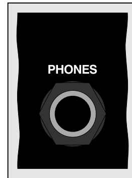
Figure 4. Detail of back panel showing 2-channel (stereo) headphone output jack
