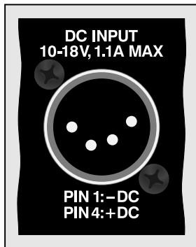
Figure 6. Detail of back panel showing the DC input power connector
