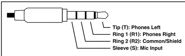
Figure 3. Headset B (TRRS) connection pinout chart
