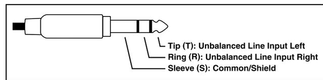
Figure 4. Stereo line in (TRS) connection pinout chart
