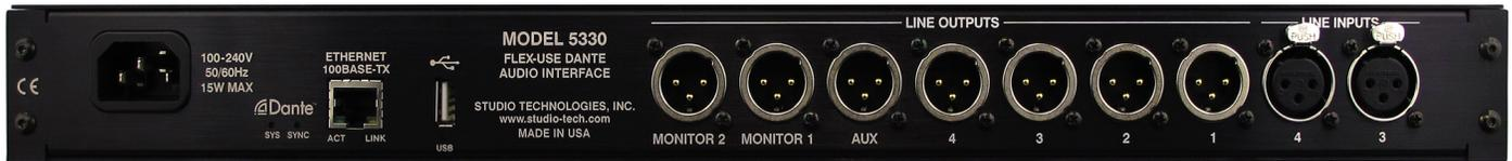
An Ethernet connection is all that's required to make the Model 5330 part of a sophisticated networked audio system. Dante audio-over-Ethernet has found wide acceptance as an audio "backbone" due to its ease of use, interoperability, excellent audio quality, and wide adoption by a large number of equipment manufacturers.
