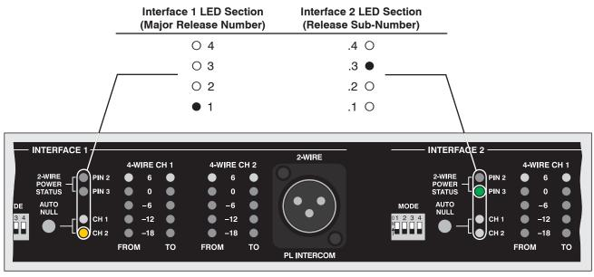
Figure 12. Detail of front panel showing the status LEDs that display the software version. In this example, the software version is 1.3.
