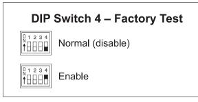
Figure 10. DIP Switch 4—Factory Test
