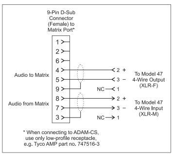
ADAM<sup>™</sup> Matrix Intercom System Analog Ports to Model 47 Interface
