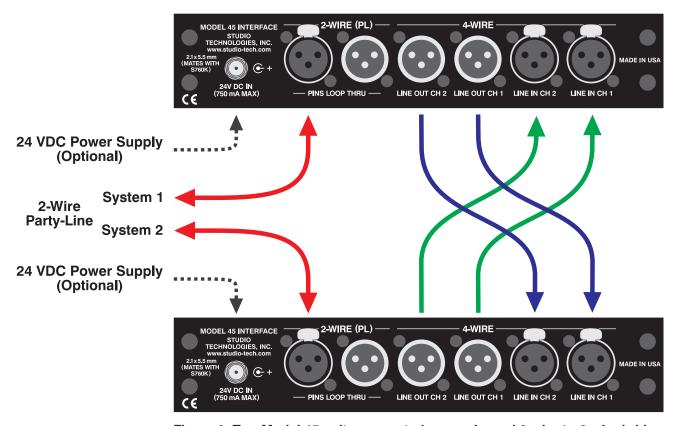
Figure 9. Two Model 45 units connected as a universal 2-wire-to-2-wire bridge
