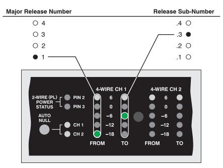
Figure 8. Detail of front panel showing the status LEDs that display the software version. In this example, the software version is 1.3.
