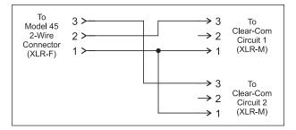
Figure 5. Adapter cable wiring diagram
