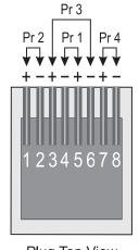
Plug Top View (Release Tab on Bottom)
