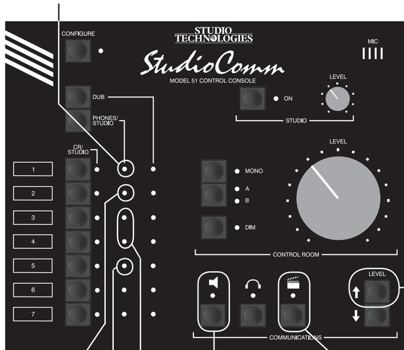
Press and hold Phones/Studio, then press CR/Studio 2 to toggle between normal dub source and dub follows control room source; LED on means dub follows control room
