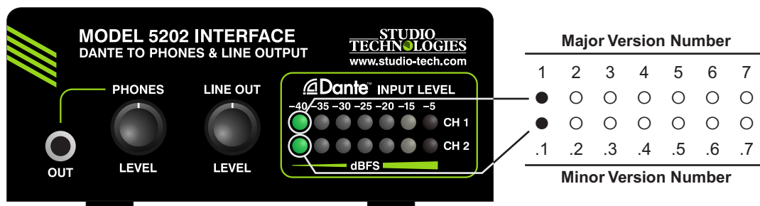
Figure 2. Detail of front panel showing the LEDs that display the firmware version. In this example, the version shown is 1.1.
