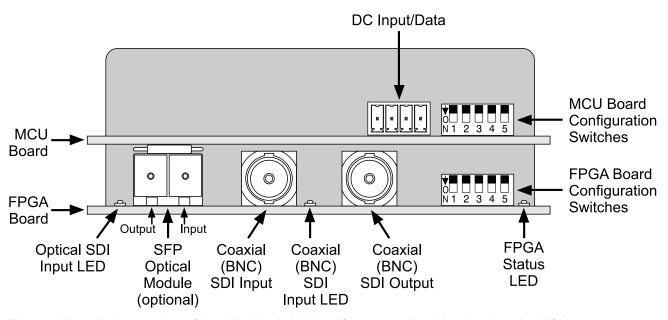
Figure 2. Detailed rear view of the Model 5150 Video Generator Module showing the MCU and FPGA boards
