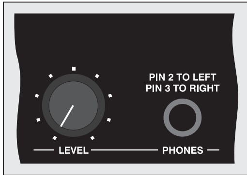
Figure 8. Detail of front panel showing headphone section
