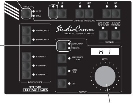
Use the Level control to change this specific **Model 77's device address**. Address can be either A1, A2, A3, or A4.
