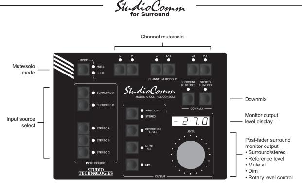
Figure 3. Model 77 Control Console Front Panel
