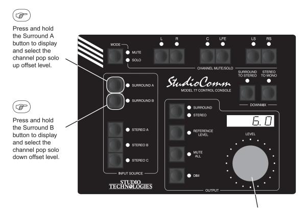
When the Surround A button is pressed, use the level control to adjust the **channel pop solo up offset level**. The range is 0.0 to 12.0 in 0.5-dB steps.
