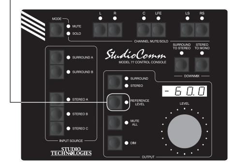
Default: Reference level set for -60.0 dB post-fader monitor output level.
