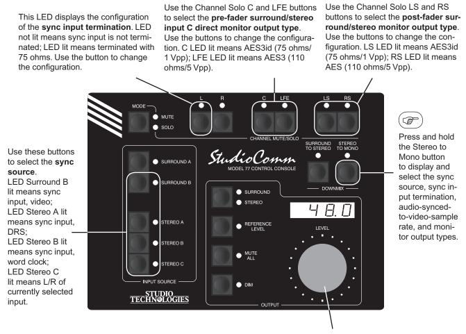
Use the level control to adjust the **audiosynced-to-video sample rate**. Available sample rates are 32, 44.1, 48, 88.2, 96, 176.4, and 192 kHz.
