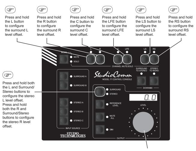
Use the level control to adjust the **post-fader monitor output level offsets**. The range is -12.0 to 12.0 in 0.5-dB steps.
