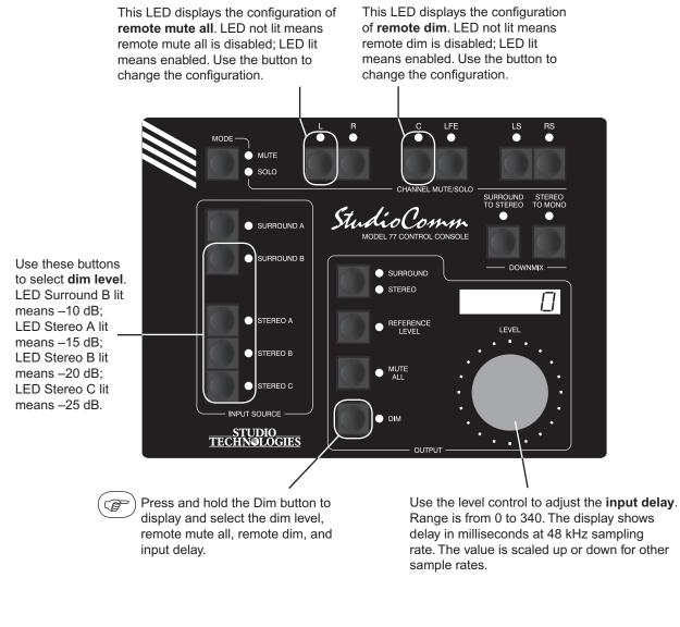
Default: -20 dB dim level. Remote mute all enabled. Remote dim enabled. Input delay 0 ms.
