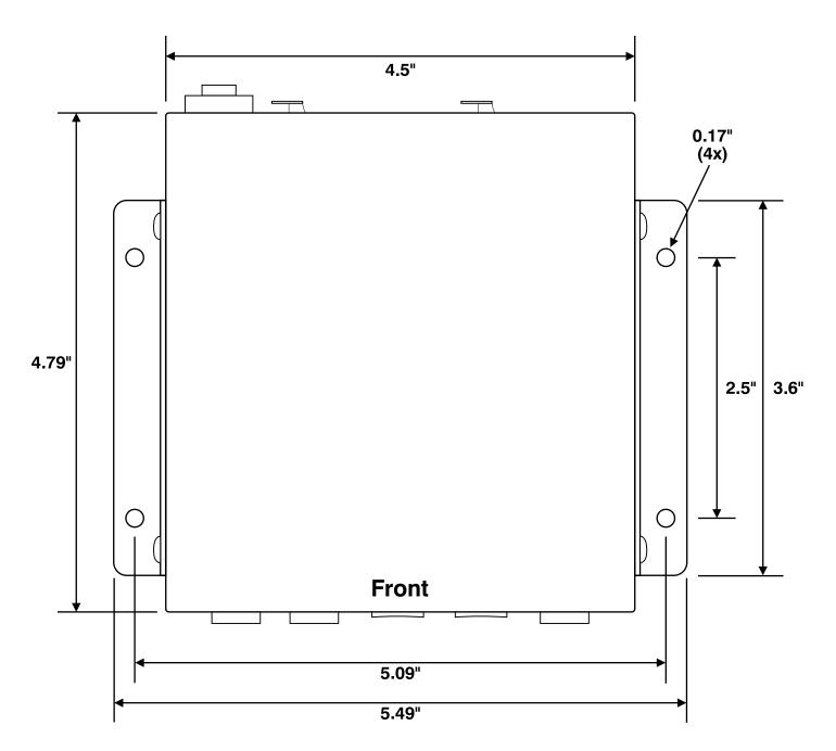
Overall Height with Brackets Installed = 1.63"
