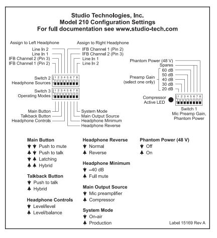
Model 210 configuration settings label as affixed to security plate Actual size 4.25" x 4.60" Cut along lines for use as a spare
