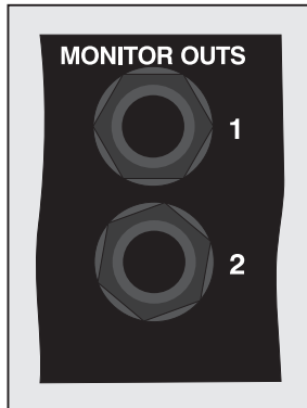
Figure 6. Detail of back panel showing monitor output connectors
