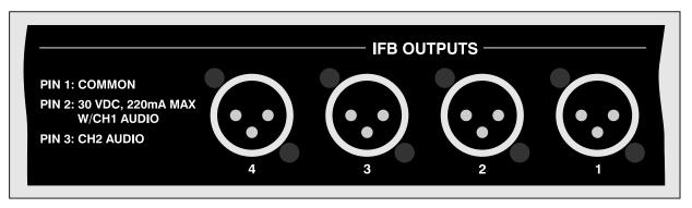
Figure 5. Detail of back panel showing IFB output connectors
