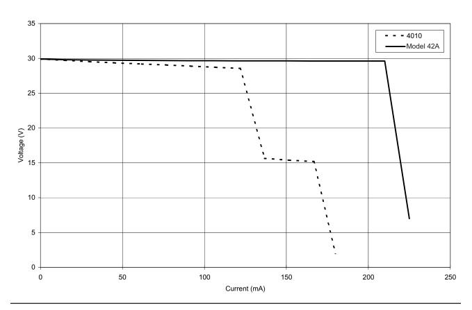
Figure 10. IFB output voltage-current curves for RTS 4000-Series and Model 42A Interface
