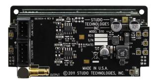
Model 5110 Mic/Line Input Module Back View
