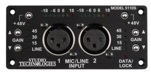
Model 5110S Mic/Line Input Module Front Panel
