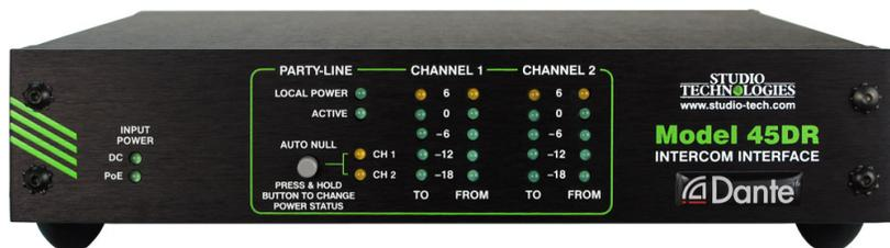
the Model 45DR, allowing connection of user belt-packs such as the popular RTS BP-325. A Model 45DR can also connect with an existing powered and terminated intercom circuit. Audio level meters provide confirmation of system performance during setup and operation. Support for transporting call light signals between Model 45DR units is also provided.
