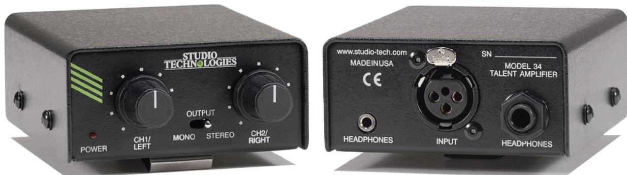
The Model 34 is compatible with virtually every standard broadcast IFB and party-line intercom circuit. This type of circuit typically uses 3-pin XLR-type connectors for interfacing with connected equipment. XLR pin 1 serves as common for DC power and audio. Pin 2 provides DC power and, in the case of a dual-channel circuit, DC power and channel 1 audio. Pin 3 provides channel 2 audio in dual-channel systems or channel 1 audio in single-channel systems.
