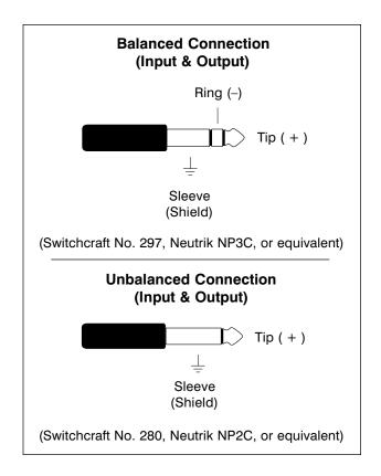
**Caution:** For reliable audio interconnection, the plugs you use must comply with industry standard RS-453. Switchcraft No. 297, Neutrik NP3C, or equivalent will work correctly. Refer to the Technical Notes section for details.
