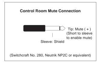
Access to the control room mute function is via a ¼-inch jack located on the Model 60's back panel. Mute is enabled whenever the tip lead is shorted (connected) to the sleeve lead. Using a ¼-inch phone plug, connect a normally open contact to the tip and sleeve. The contact must be capable of handling a current of 7 milliamperes at 15 volts DC.
