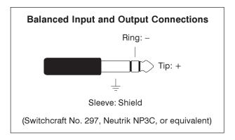
an unbalanced source connect the tip to high (+ or hot), and both the ring and sleeve to shield. If connecting to an unbalanced source in this manner results in hum or noise, connect tip to high (+ or hot) and ring to shield; leave the sleeve unterminated.
