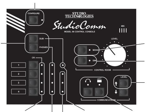
Press Mono to toggle between latching or momentary operation; LED on means the Mono button is set to latch
