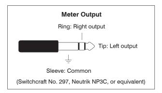
a nominal level of +4dBu, and is capable of driving loads of 2k ohms and greater. A 1/4-inch 3-conductor plug should be wired with tip for the left output, ring for the right output, and sleeve for common.
