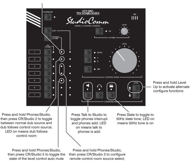
Press and hold Phones/Studio, then press CR/Studio 5 to toggle the state of the level control auto mute function; when the LED is lit the function is enabled
