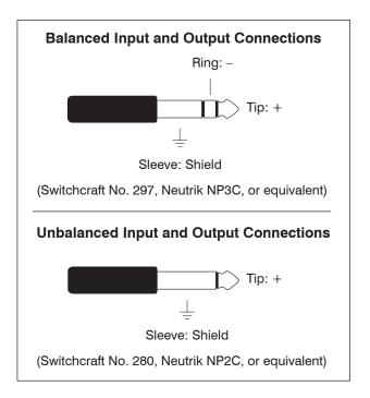
For connection of balanced input and output signals, ¼-inch 3-conductor phone plugs should be used. The plugs should be wired with tip positive (+ or hot), ring negative (- or cold), and sleeve shield. With unbalanced input and output signals, either ¼-inch 2- or 3-conductor plugs can be used. With 2-conductor plugs tip should be wired as positive (+ or hot) and sleeve as shield. With 3-conductor plugs tip should be wired as positive (+ or hot) and both ring and sleeve as shield.
