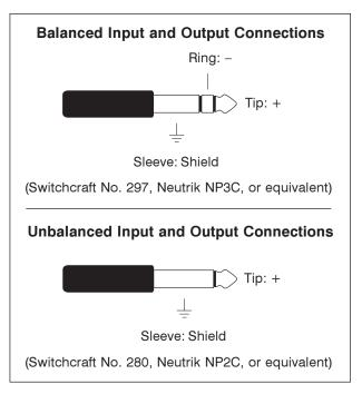
For connection of balanced input and output signals, 1/4-inch 3-conductor phone plugs should be used. The plugs should be wired with tip positive (+ or hot), ring negative (- or cold), and sleeve shield. With unbalanced input and output signals, either 1/4-inch 2- or 3-conductor plugs can be used. With 2-conductor plugs tip should be wired as positive (+ or hot) and sleeve as shield. With 3-conductor plugs tip should be wired as positive (+ or hot) and both ring and sleeve as shield.
