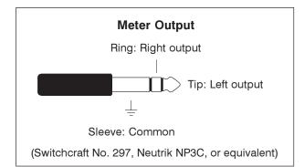
driving loads of 2k ohms and greater. A <sup>1</sup>/<sub>4</sub>-inch 3-conductor plug should be wired with tip for the left output, ring for the right output, and sleeve for common.
