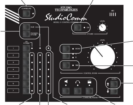
Press Mono to toggle between latching or momentary operation; LED on means the Mono button is set to latch
