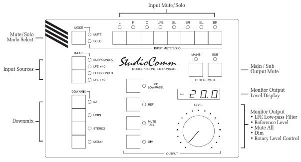
**Model 79 Control Console Front Panel**
