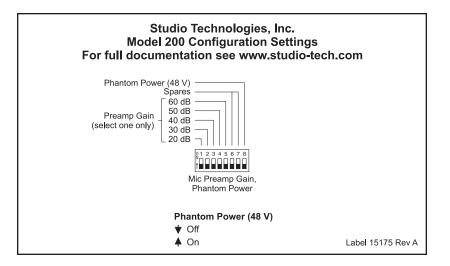
Model 200 configuration settings label as affixed to security plate Actual size 4.25" x 2.50" Cut along lines for use as a spare
