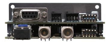
Model 5152 Video Generator/Audio Embedder Module Back View
