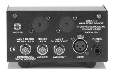
interface is transformer-coupled and capable of driving long broadcast cable runs.
