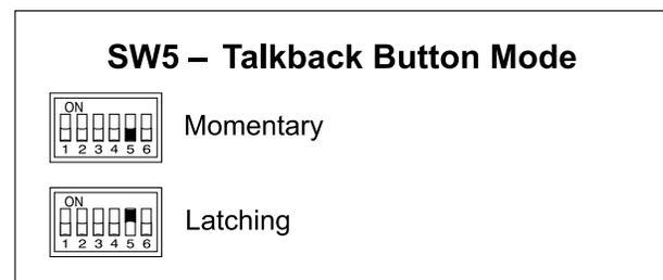
**Figure 4. Talkback button mode configuration switch**
