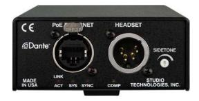
interface with twisted-pair Ethernet local-area-networks using standard RJ45 patch cables. This LAN connection provides both Power-over-Ethernet (PoE) and bidirectional digital audio signals.
