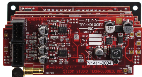
Figure 1. Model 5110S Mic/Line Input Module front and back views (serial numbers 151-200 shown)
