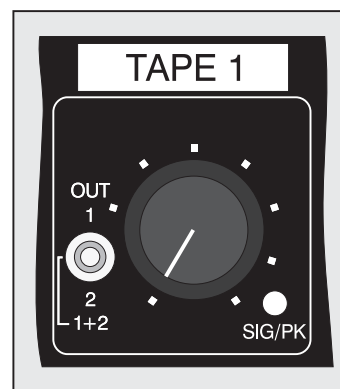
Detail of front panel showing installation-specific label
