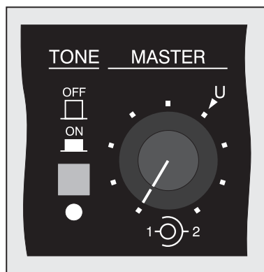
Detail of front panel showing master level controls, reference tone on/off button, and reference tone active LED
