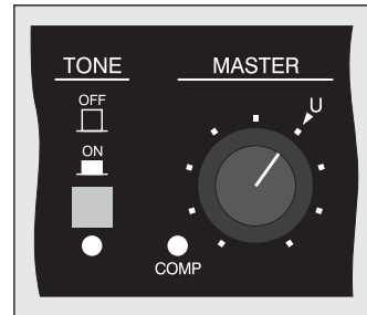
Detail of front panel showing master level control, compressor active LED, and reference tone on/off button
