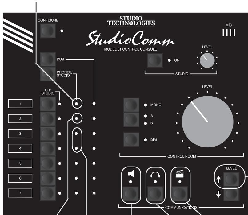
Press and hold Level Up to activate alternate configure functions
