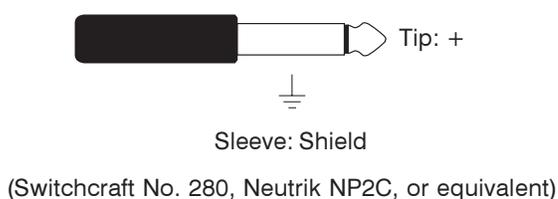
For connection of balanced input and output signals, 1/4-inch 3-conductor phone plugs should be used. The plugs should be wired with tip positive (+ or hot), ring negative (- or cold), and sleeve shield. With unbalanced input and output signals, either 1/4-inch 2- or 3-conductor plugs can be used. With 2-conductor plugs tip should be wired as positive (+ or hot) and sleeve as shield. With 3-conductor plugs tip should be wired as positive (+ or hot) and both ring and sleeve as shield.
