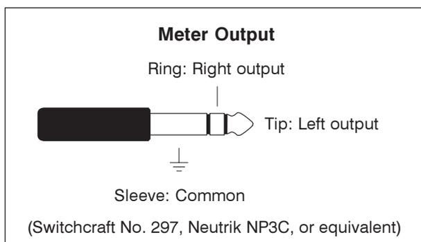
driving loads of 2k ohms and greater. A 1/4-inch 3-conductor plug should be wired with tip for the left output, ring for the right output, and sleeve for common.
