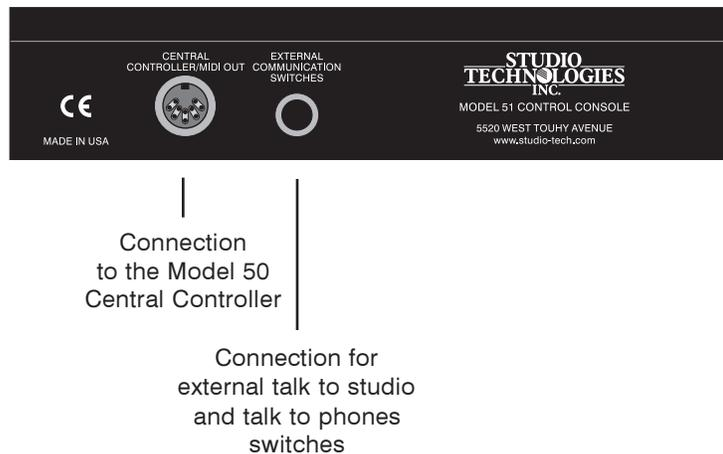
Four functions can be set for push-to-latch operation if desired: talk to studio, talk to phones, slate, and control room mono.
