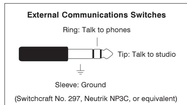
to phones access even when external switches are connected.
